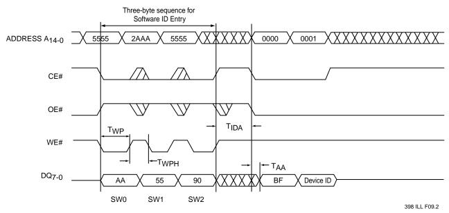
Device ID = B5H for SST39SF010A, B6H for SST39SF020A, and B7H for SST39SF040
