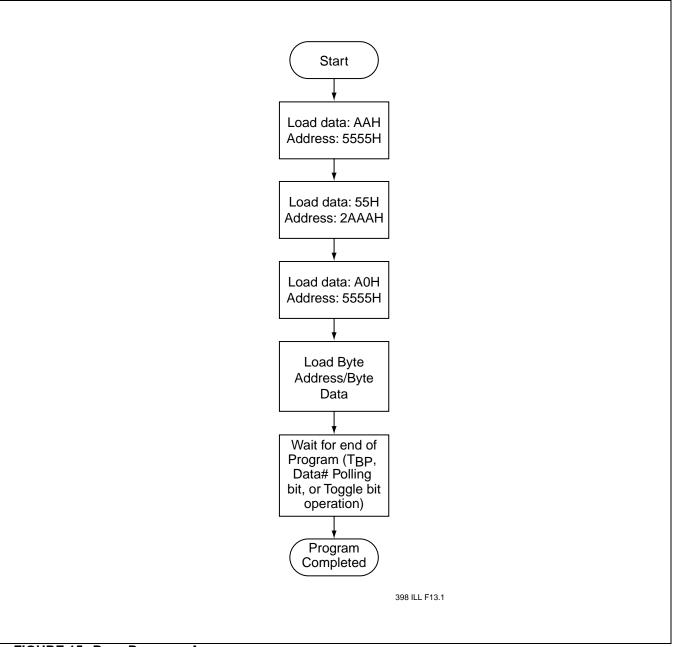
FIGURE 15: BYTE-PROGRAM ALGORITHM
