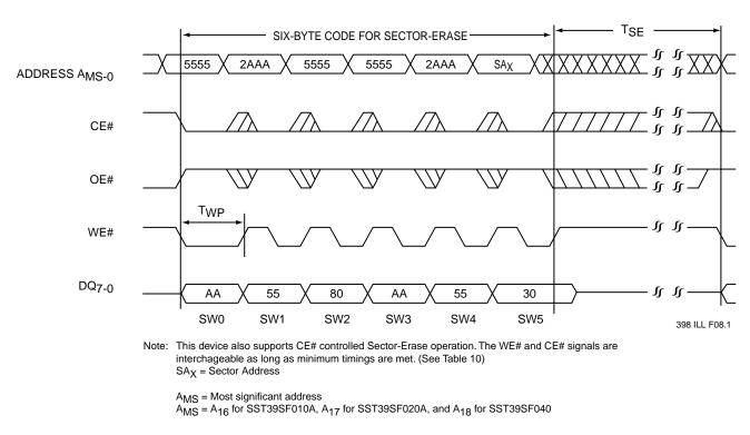
FIGURE 9: WE# CONTROLLED SECTOR-ERASE TIMING DIAGRAM
