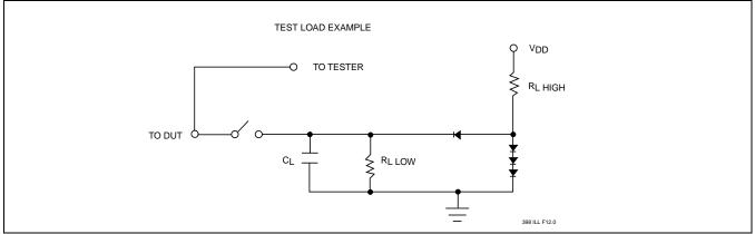
FIGURE 14: A TEST LOAD EXAMPLE
