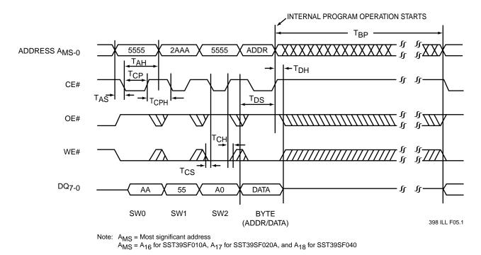
FIGURE 6: CE# CONTROLLED PROGRAM CYCLE TIMING DIAGRAM
