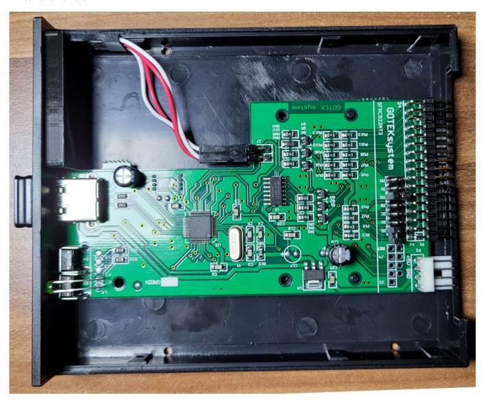
To flash the Gotek you need the special USB cable with USB-A connectors on both ends. Before connecting the USB cable you need to short the Boot (J3) jumper in order to disable the old firmware and let the computer detect the device for flashing. As the jumper pins are not installed by default, you may need to use a wire to short the 2 leftmost pads on the circuit board:
