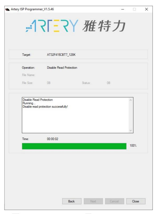
Click Back and choose "Download to device". Then click Add and select the previously unpacked FlashFloppy firmware file in HEX format: FF\_Gotek-v3.24.hex (please use version 3.24 or later!). Don't forget to check the "Verify after download" option. You can enable the read protection by checking the "Enable Read Protection after Download" option, but then you won't be able to verify the uploaded firmware. Before flashing the interface will look like that:
