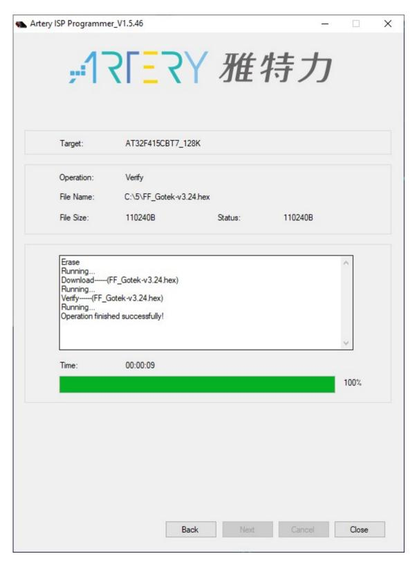
Basically, that's it. We just need to disconnect the Gotek from the USB cable and to connect the power to its power connector. If you see the "F-F" letters (or "FlashFloppy" with version number in case you installed an OLED screen), then the firmware has been uploaded successfully. If you need to change the firmware or upload it again, you need to set the jumper once more to prevent the firmware from starting before connecting the USB cable to the Gotek.
