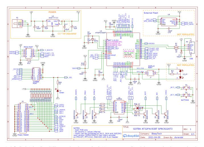
And, finally, let's install an OLED screen into the new Gotek. It's no more complicated than connecting the screen into the older Gotek version. More information can be found here. The wiring for connecting an OLED screen to the new Gotek's board looks like this:
