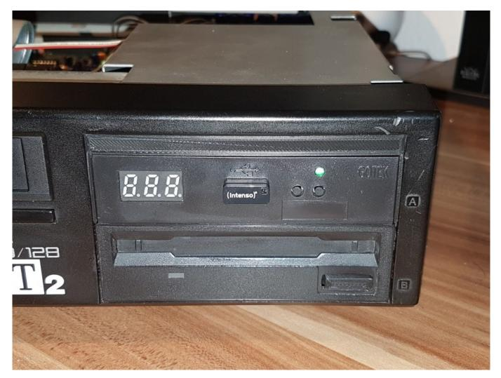
After installation please power up the computer and check that you can boot from the mounted DSK image located on the USB drive. If the computer only boots to MSX Basic, use the files command to list the directory of the mounted DSK image. If the image is not mounted, please check whether the Gotek emulator is properly powered and connected to the motherboard. Also check that the mounted DSK image is good.
