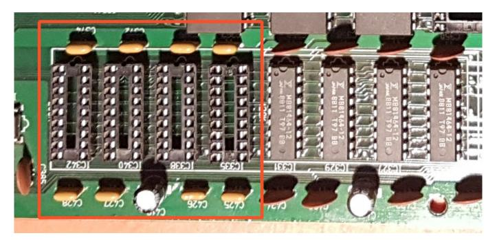
Then you need to install 8 ceramic 100nF capacitors on C425, C426, C427, C428, C363, C365, C372 and C374 placeholders and also add one electrolytic 100uF 16v capacitor on C419 placeholder. Please mind the capacitor's polarity when installing it. Then you can insert 4 DRAM chips into the sockets. The chips must be x464 DRAM with speeds from 80 to 120ns. The fully upgraded RAM looks like that:
