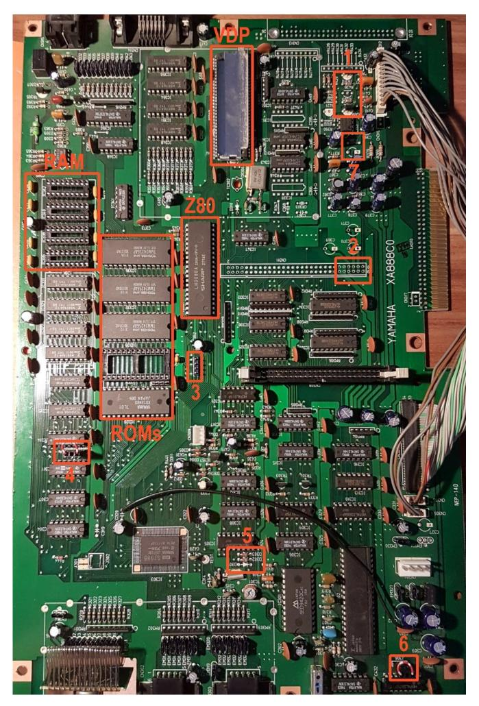
The v9958 VDP must be installed onto the motherboard first. The older VDP (v9938) must be removed. The initial step is to desolder and remove the heatsink that is located on top of the VDP chip. The heatsink has 2 solder points on the motherboard near the narrow chip's edges. On the below picture they are shown in red frames. Those points need to be heated so that the heatsink could be easily removed. Be careful not to cut your fingers with the sharp edges!
