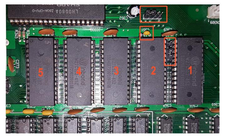
To complete the job you need to program 5 ROM chips with the necessary data using any EEPROM programmer. We recommend to use only the electrically erasable W27C512 EEPROM chips from Winbond. The chips on the above image are marked as 1,2,3,4 and 5. You need to write the data from the files with the corresponding names into the chips and put them into the sockets according to their numbering. The archive with the data is located here.
