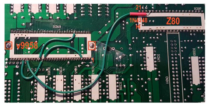
The new VDP could be installed into a socket, but we recommend to solder it directly onto the motherboard in order to prevent poor connection during the prolonged use. The new VDP has a slightly different pinout, so a few wires need to be soldered between the following pins:
