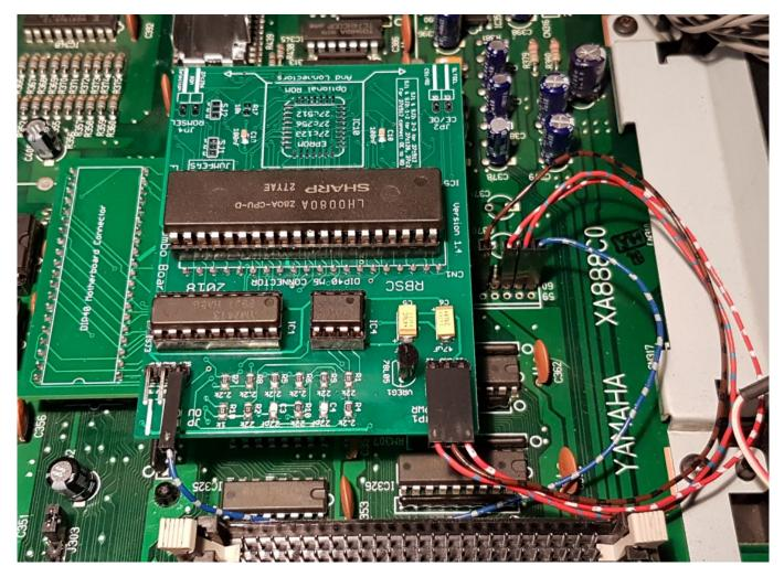
To enable sound output from the FMPAC/F4 combo board to the internal amplifier please solder a 4.7kOhm resistor to the placeholder marked as "R381" and a 4.7uF 50V electrolytic capacitor to the placeholder marked as "C397". Mind the polarity
