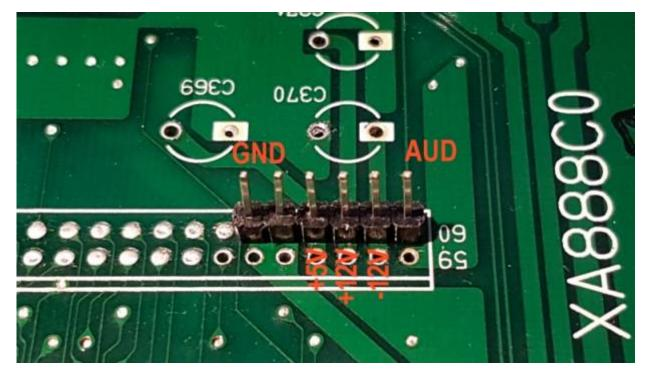
The assembled combo board (without the ROM chip) is installed into the socket of the adapter board by gently pushing it downwards. Please make sure that the pins of the combo board are connected to the socket in the right way or you may damage the Z80 CPU installed on the board. The picture below shows how the combo board is installed and connected to the newly-soldered pins on the motherboard.
