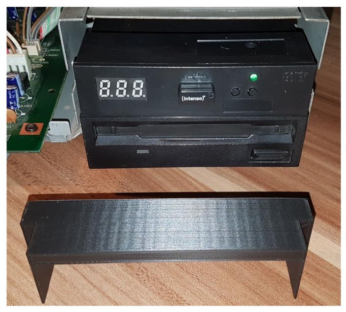
The 3D-printed part is installed on top of the Gotek's case, then the front panel is attached to the MSX's case so that there are no gaps between the emulator's case and the front panel. See the below picture for reference.
