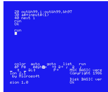
TEXT1 mode, horizontal scan line is 240 dots, garbage in un-initialized memory space
