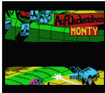
Offset screen*, horizontal scan line is 256 dots, GRAPHIC1 mode, top appears at the bottom
